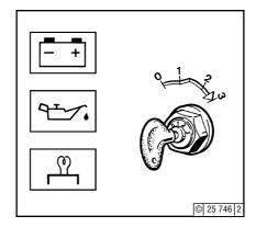
Turn key anticlockwise (to position 0) and remove. Pilot lights will go out.
