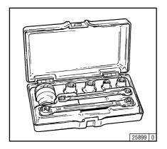
A TORX BN. 8189 screw set is used with engines in the 1011 series.
