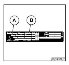
The model  ${\bf A}$ , the engine serial number  ${\bf B}$  and the performance data are stamped on the rating plate.
