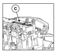
The rating plate  ${\bf C}$  is attached to the valve cover.
