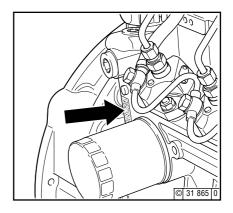
The engine serial number  ${\bf B}$  is stamped on the crankcase  ${\bf D}$  as well as the rating plate.
